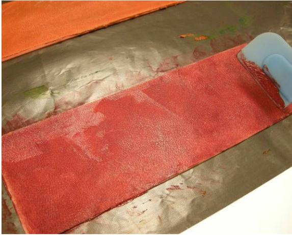
Fig. 4. The acrylic blend is applied to the silicone mold with a wide spatula to create a uniform film.
