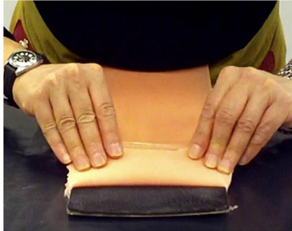
Fig. 3. The silicone mold is peeled away from the leather.
